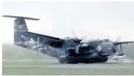
XC-8A Aircraft flight tests Bell Air Cushion Landing System at Wright-Patterson AFB (1975)
